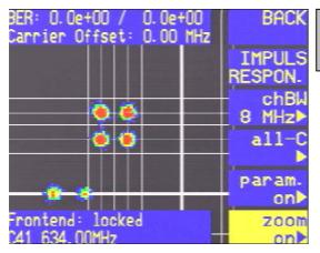
zoom on► Press this button to enlarge the constellation diagram. The upper left-hand section of the constellation diagram is now represented and allows a closer look of
